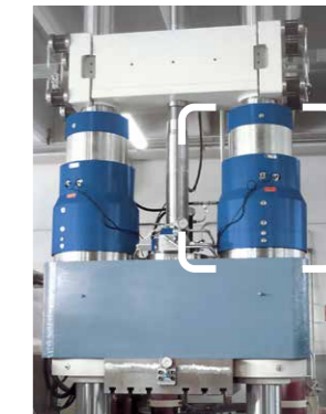
Hydraulic internal high-pressure press Generating 400 metric tons closing force
