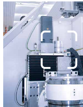
Grinding machine Securing the Z-axis in case of emergency stop and for maintenance
